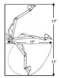
The TRUCKHOE's 17' reach and 11' digging depth are more than many tractor-mounted hoes offer.
